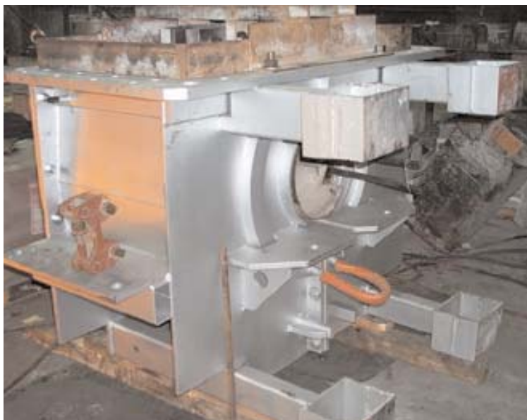
The Electric Vibration System is shown with a channel form and bushing mounted to the inductor. A temporary metal retainer is shown, as well.
