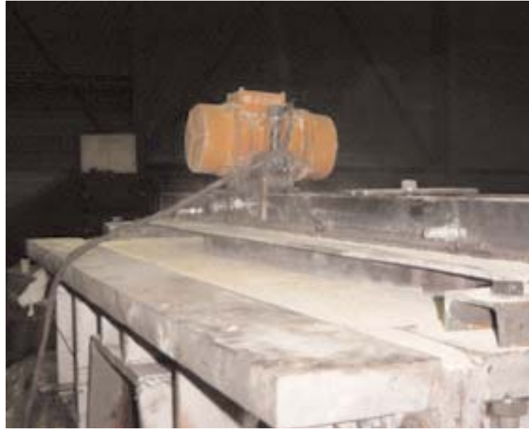
The EVS vibrator unit is shown attached to the inductor case.
