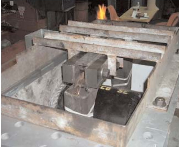
Another view of the EVS with a channel form and bushing fixed to the inductor.
